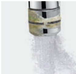
Scale build-up on aerator causes splashing
